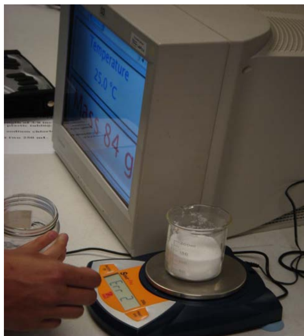
Measuring sodium-chloride by mass, a student with low vision is using a magnification program to enlarge the mass readout in the LoggerPro software from the Scout Pro scale
