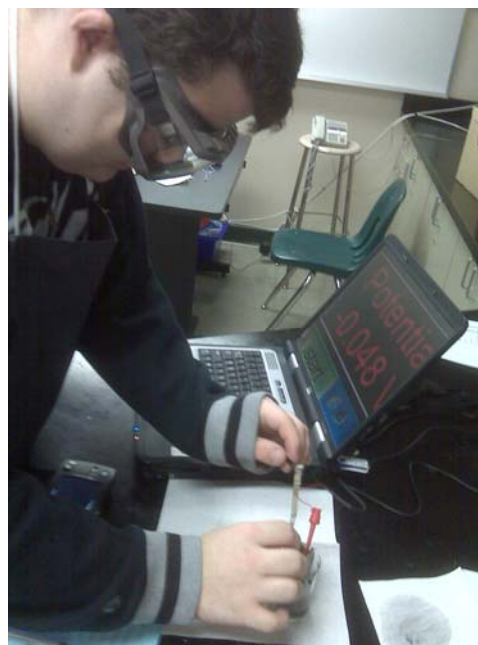
The Vernier voltage probe, connected to a laptop and used with a magnification program for the student to read the data
