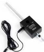
With hook for connecting to a string and measuring pulling force
